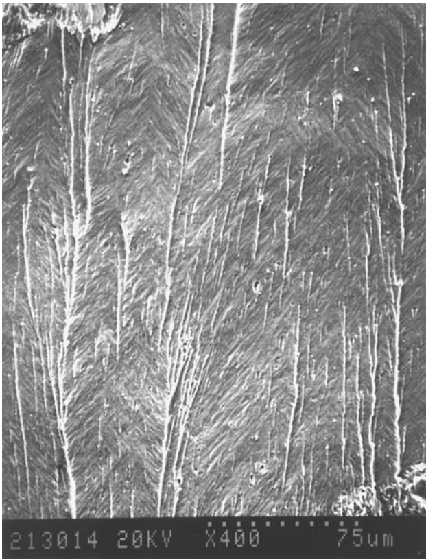
Fig. 21 River patterns in R2 pre-crack region, LR orientation (400×)
