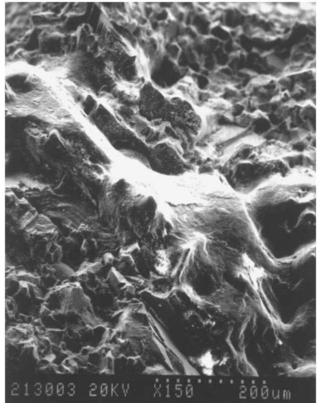
Fig. 17 Black dots in R1 pre-crack region, LC orientation (150×)
