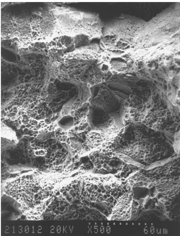
Fig. 19 Transgranular dimples with some cleavages in R2 pre-crack region, CR orientation (500×)
