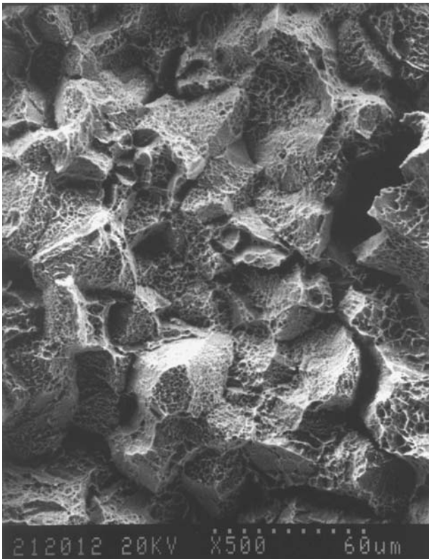
Fig. 16 Dimples in R1 fracture region, LR orientation (500×)
